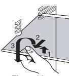
• The glass shelves are **Figure 29** fitted with stops to prevent them from being pulled out accidentally.
